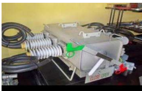
Gambar 2. Load Break Switch (LBS)
