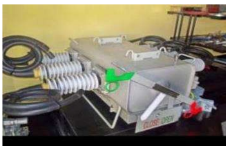
Gambar 2. Load Break Switch (LBS)
